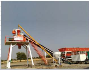
STATIONARY BATCHING PLANT Capacity 20 To 120 M3/Hr
