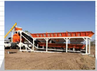
INLINE MOBILE BATCHING PLANT WITH TWIN SHAFT MIXER Capacity 20,30 M3/hr
