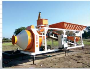
REVERSIBLE BATCHING PLANT Capacity 20 M3/Hr
