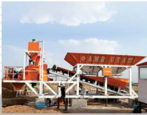
NANO MOBILE BATCHING PLANT Capacity 20,24 M3/Hr
